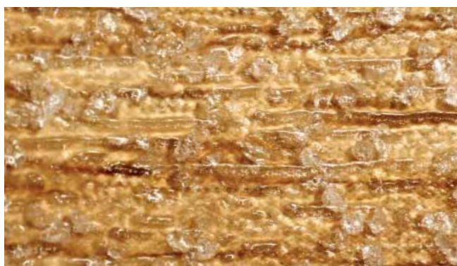
Magnification showing aggregates within Polysafe Wood FX product.
